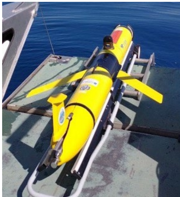
Figure 39. The UC Davis glider being recovered from Lake Tahoe with the equipped science payload.
