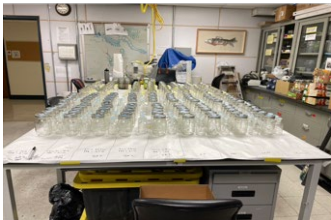
Figure 13. Left: incubations bottles for dissolved oxygen PreSens sensors and 14C method in the lab at the University of Nevada Reno, and right: Dr. Steve Sadro leads a team to fill incubation bottles with lake water from Lake Tahoe and Castle Lake.
